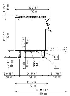
Electrical inlet (power) Gas connection
